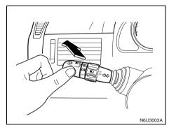
To change the headlamps from low beam to high beam, push the turn signal multi-function lever away from you.
